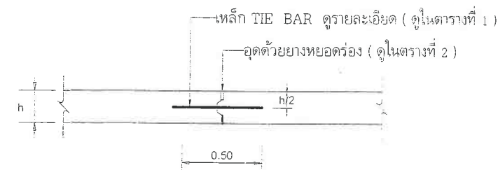
LONGITUDINAL JOINT SCALE 1 : 25
